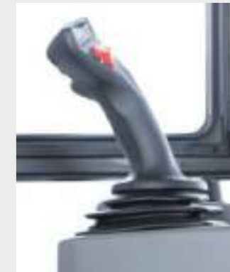
Control & operating elements: Reduced elements for intuitive operation, joystick moves ergonomically with the seat and fits any hand size
