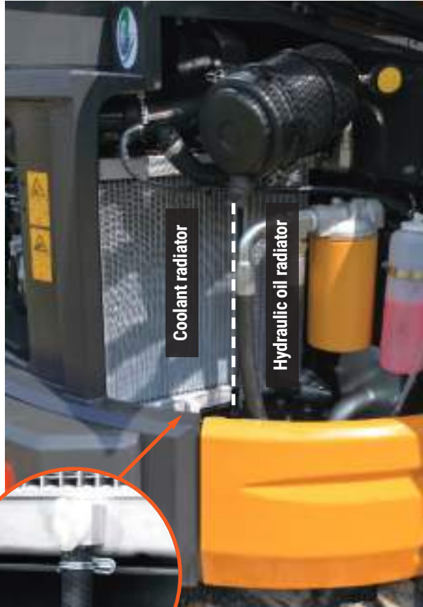
Cooling and supply air intake
