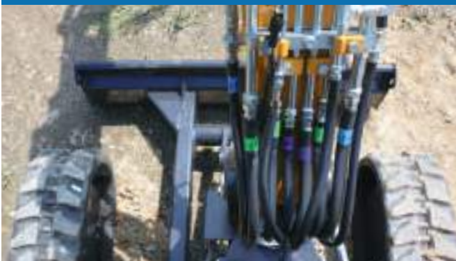
Well arranged hydraulic pipes - good visibility of the digging area
