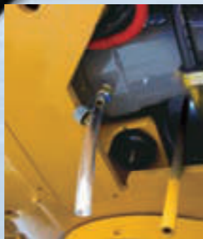
▲ The one touch cock enables to discharge oil without staining hand or using tool.
