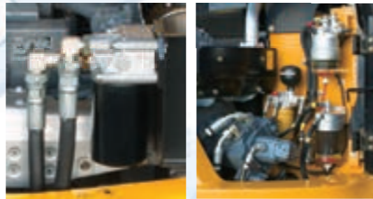
▲ Easy access to the fuel filter and the engine oil filter.
