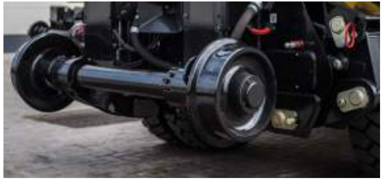
As option available: Friction Drive System available for 1404 ZW with track width 1000 and 1435 mm..
