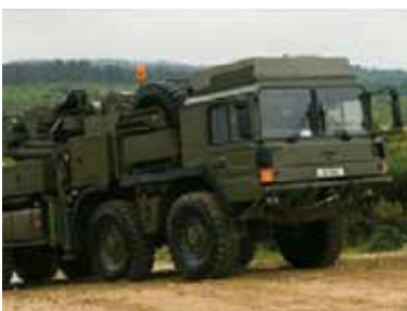
MAN Recovery unit with 600.2 crane
