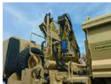
Folded 165M1 crane fitted to SLDT(P)
