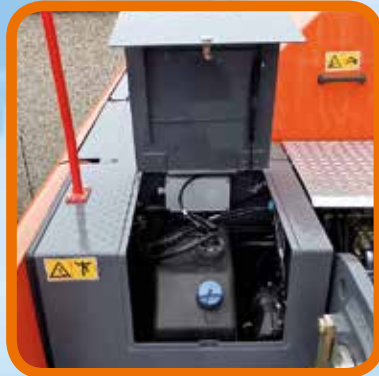
Easily accessible AdBlue® tank
