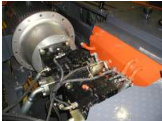
E-drive and main pumps
